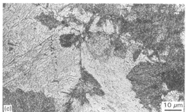
Figure 5 Microstructure of Ni26MoTi2Nb steel: (a) after cold treating, (b, c) after three repeated heatings to 999.9 K at a rate of (b) 2.5 K min -1 and (c) 40 K min -1 .
